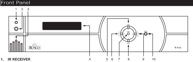
Receives the infrared signal from the remote control.
